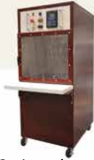
Corriente alterna, 20 kV, ASTM D149
